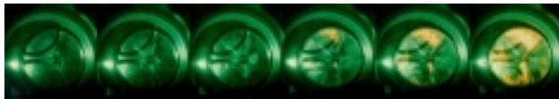
Figure D2.7.2. A sequence of stills from a high speed movie of diesel fuel injection. Taken with a film camera and copper vapour laser illumination. Courtesy K.K. Rao.
